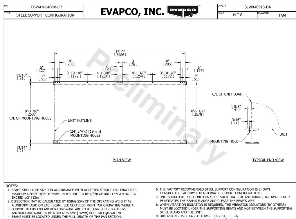
SUPPORTING BEAM SURFACE MUST BE LEVEL. DO NOT LEVEL THE UNIT BY PLACING SHIMS BETWEEN THE UNIT MOUNTING FLANGE AND THE SUPPORTING BEAM. [METRIC] [mm]
