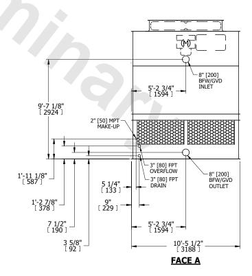
DRAWN BY: JLG NO. OF SHIPPING SECTIONS **SHIPPING** OPERATING HEAVIEST SECTION 5550 lbs+ [2520] kg+ 8850 lbs+ [4015] kg+ 3950 lbs+ [1795] kg+ WEIGHT WEIGHT WEIGHT
