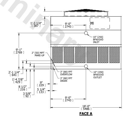
DRAWN BY: KDS NO. OF SHIPPING SECTIONS **SHIPPING** OPERATING HEAVIEST SECTION 10710 lbs+ [4860] kg+ 19980 lbs+ [9065] kg+ 6810 lbs+ [3090] kg+ WEIGHT WEIGHT WEIGHT
