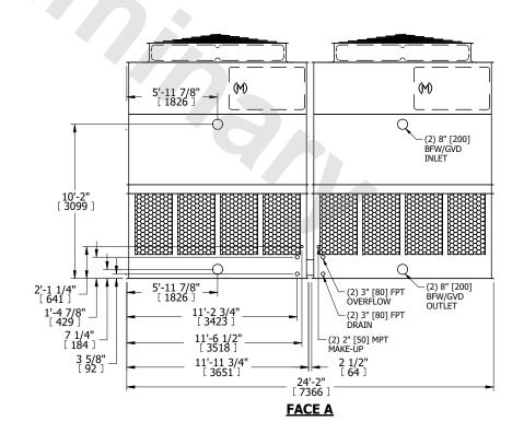
SHIPPING WEIGHT 16260 lbs+ [7380] kg+ OPERATING WEIGHT 28680 lbs+ [13010] kg+ HEAVIEST SECTION WEIGHT 5590 lbs+ [2540] kg+ NO. OF SHIPPING SECTIONS 4 DRAWN BY: KDS
