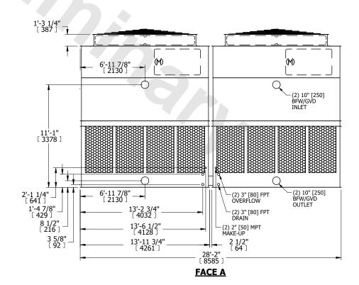
SHIPPING WEIGHT 18400 lbs+ [8350] kg+ OPERATING WEIGHT 33060 lbs+ [15000] kg+ HEAVIEST SECTION WEIGHT 6150 lbs+ [2790] kg+ NO. OF SHIPPING SECTIONS 4 DRAWN BY: KDS
