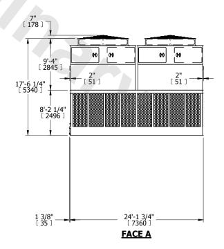
SHIPPING WEIGHT 34540 lbs+ [15670] kg+ OPERATING WEIGHT 58860 lbs+ [26700] kg+ HEAVIEST SECTION WEIGHT 5790 lbs+ [2630] kg+ NO. OF SHIPPING SECTIONS 6 DRAWN BY: JLG
