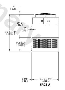
SHIPPING WEIGHT 15640 lbs+ [7095] kg+ OPERATING WEIGHT 25560 lbs+ [11595] kg+ HEAVIEST SECTION WEIGHT 5370 lbs+ [2440] kg+ NO. OF SHIPPING SECTIONS 4 DRAWN BY: JLG
