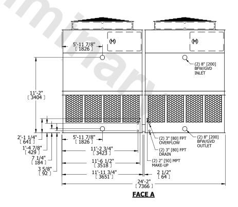
SHIPPING WEIGHT 17240 lbs+ [7820] kg+ OPERATING WEIGHT 29660 lbs+ [13455] kg+ HEAVIEST SECTION WEIGHT 6080 lbs+ [2760] kg+ NO. OF SHIPPING SECTIONS 4 DRAWN BY: KDS
