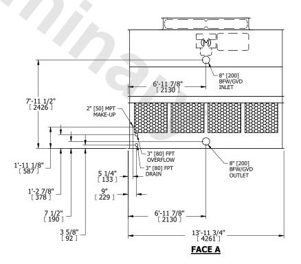
SHIPPING WEIGHT 5880 lbs+ [2670] kg+ OPERATING WEIGHT 10390 lbs+ [4715] kg+ HEAVIEST SECTION WEIGHT 3830 lbs+ [1740] kg+ NO. OF SHIPPING SECTIONS 2 DRAWN BY: JLG
