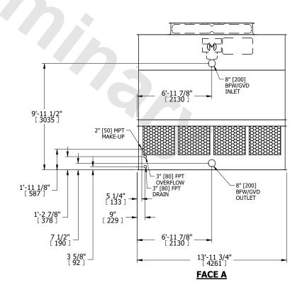
SHIPPING WEIGHT 6780 lbs+ [3080] kg+ OPERATING WEIGHT 11290 lbs+ [5125] kg+ HEAVIEST SECTION WEIGHT 4730 lbs+ [2150] kg+ NO. OF SHIPPING SECTIONS 2 DRAWN BY: JLG
