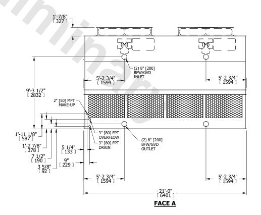
DRAWN BY: JLG SHIPPING NO. OF SHIPPING SECTIONS OPERATING HEAVIEST SECTION 10210 lbs+ [4635] kg+ 17150 lbs+ [7780] kg+ 7020 lbs+ [3185] kg+ WEIGHT WEIGHT WEIGHT
