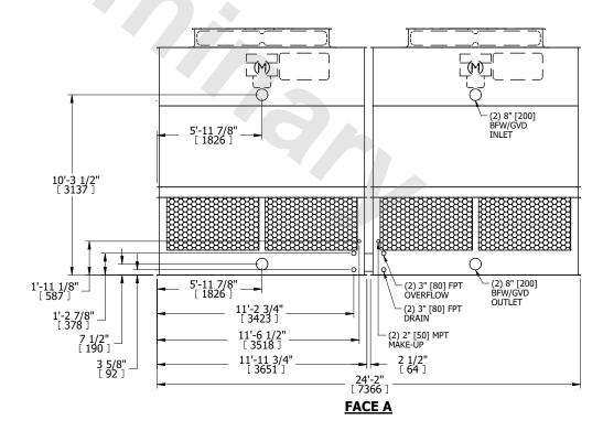
SHIPPING WEIGHT 12380 lbs+ [5620] kg+ OPERATING WEIGHT 20100 lbs+ [9120] kg+ HEAVIEST SECTION WEIGHT 4330 lbs+ [1965] kg+ NO. OF SHIPPING SECTIONS 4 DRAWN BY: JLG
