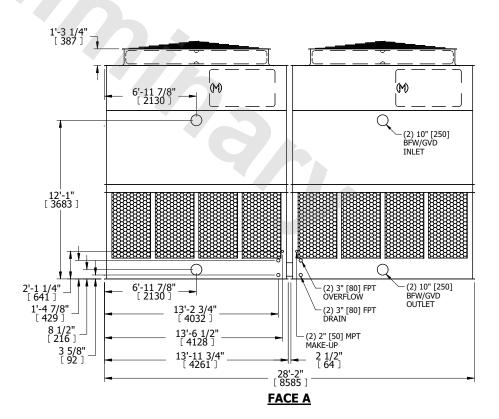
SHIPPING WEIGHT 19560 lbs+ [8875] kg+ OPERATING WEIGHT 34220 lbs+ [15525] kg+ HEAVIEST SECTION WEIGHT 6730 lbs+ [3055] kg+ NO. OF SHIPPING SECTIONS 4 DRAWN BY: KDS
