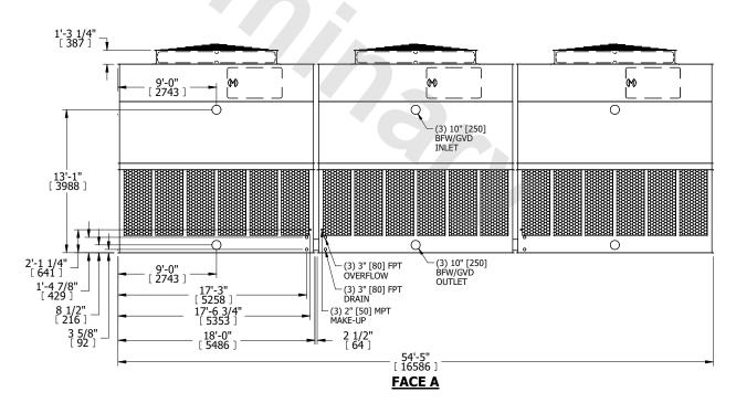
SHIPPING WEIGHT 39150 lbs+ [17760] kg+ OPERATING WEIGHT 66960 lbs+ [30375] kg+ HEAVIEST SECTION WEIGHT 8870 lbs+ [4025] kg+ NO. OF SHIPPING SECTIONS 6 DRAWN BY: KDS
