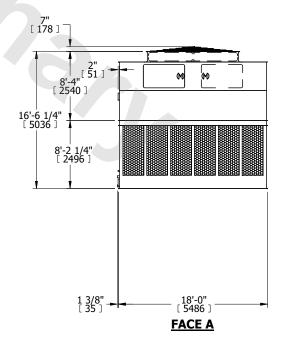
SHIPPING WEIGHT 22600 lbs+ [10255] kg+ OPERATING WEIGHT 41140 lbs+ [18665] kg+ HEAVIEST SECTION WEIGHT 6920 lbs+ [3140] kg+ NO. OF SHIPPING SECTIONS 4 DRAWN BY: KDS
