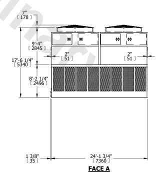
DRAWN BY: JLG NO. OF SHIPPING SECTIONS **SHIPPING** OPERATING HEAVIEST SECTION 5790 lbs+ [2630] kg+ 33940 lbs+ [15395] kg+ 58260 lbs+ [26430] kg+ WEIGHT WEIGHT WEIGHT
