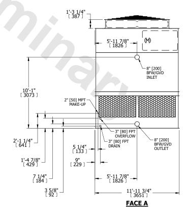
SHIPPING WEIGHT 7790 lbs+ [3535] kg+ OPERATING WEIGHT 12750 lbs+ [5785] kg+ HEAVIEST SECTION WEIGHT 5370 lbs+ [2440] kg+ NO. OF SHIPPING SECTIONS 2 DRAWN BY: JLG
