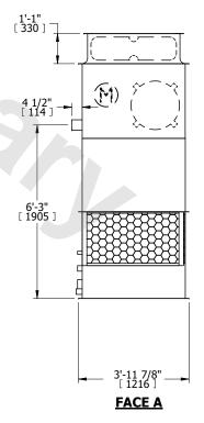
DRAWN BY: KWC NO. OF SHIPPING SECTIONS **SHIPPING** OPERATING HEAVIEST SECTION 1130 lbs+ [515] kg+ 1760 lbs+ [800] kg+ 780 lbs+ [355] kg+ WEIGHT WEIGHT WEIGHT
