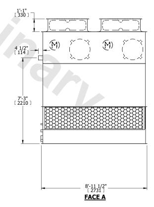
SHIPPING WEIGHT 2260 lbs+ [1030] kg+ OPERATING WEIGHT 3810 lbs+ [1730] kg+ HEAVIEST SECTION WEIGHT 1640 lbs+ [745] kg+ NO. OF SHIPPING SECTIONS 2 DRAWN BY: KWC
