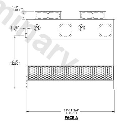
SHIPPING WEIGHT 2770 lbs+ [1260] kg+ OPERATING WEIGHT 4890 lbs+ [2220] kg+ HEAVIEST SECTION WEIGHT 2010 lbs+ [915] kg+ NO. OF SHIPPING SECTIONS 2 DRAWN BY: KWC
