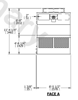
SHIPPING WEIGHT 6400 lbs+ [2905] kg+ OPERATING WEIGHT 10480 lbs+ [4755] kg+ HEAVIEST SECTION WEIGHT 2010 lbs+ [915] kg+ NO. OF SHIPPING SECTIONS 4 DRAWN BY: KDS
