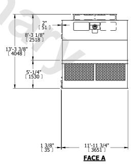
DRAWN BY: KDS NO. OF SHIPPING SECTIONS **SHIPPING** OPERATING HEAVIEST SECTION 11620 lbs+ [5275] kg+ 3960 lbs+ [1800] kg+ 19340 lbs+ [8775] kg+ WEIGHT WEIGHT WEIGHT
