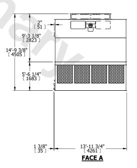
SHIPPING WEIGHT 13700 lbs+ [6215] kg+ OPERATING WEIGHT 22720 lbs+ [10310] kg+ HEAVIEST SECTION WEIGHT 4710 lbs+ [2140] kg+ NO. OF SHIPPING SECTIONS 4 DRAWN BY: KDS
