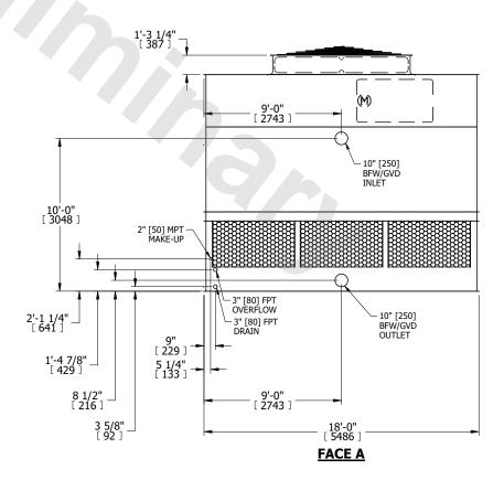
SHIPPING WEIGHT 10510 lbs+ [4770] kg+ OPERATING WEIGHT 18110 lbs+ [8215] kg+ HEAVIEST SECTION WEIGHT 6960 lbs+ [3160] kg+ NO. OF SHIPPING SECTIONS 2 DRAWN BY: KDS
