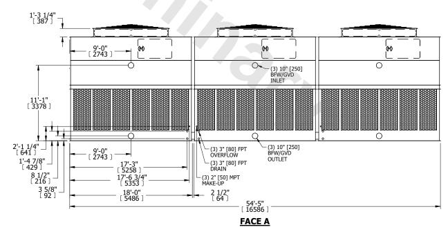
DRAWN BY: KDS NO. OF SHIPPING SECTIONS **SHIPPING** OPERATING HEAVIEST SECTION 32970 lbs+ [14955] kg+ 60780 lbs+ [27570] kg+ 6810 lbs+ [3090] kg+ WEIGHT WEIGHT WEIGHT
