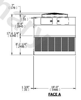
SHIPPING WEIGHT 23840 lbs+ [10815] kg+ OPERATING WEIGHT 42380 lbs+ [19225] kg+ HEAVIEST SECTION WEIGHT 7540 lbs+ [3425] kg+ NO. OF SHIPPING SECTIONS 4 DRAWN BY: KDS
