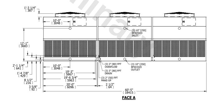
SHIPPING WEIGHT 37560 lbs+ [17040] kg+ OPERATING WEIGHT 68760 lbs+ [31190] kg+ HEAVIEST SECTION WEIGHT 8100 lbs+ [3675] kg+ NO. OF SHIPPING SECTIONS 6 DRAWN BY: KDS
