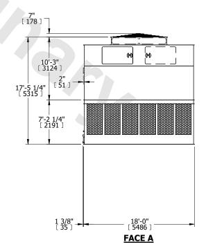
SHIPPING WEIGHT 21980 lbs+ [9970] kg+ OPERATING WEIGHT 37180 lbs+ [16865] kg+ HEAVIEST SECTION WEIGHT 7080 lbs+ [3215] kg+ NO. OF SHIPPING SECTIONS 4 DRAWN BY: KDS
