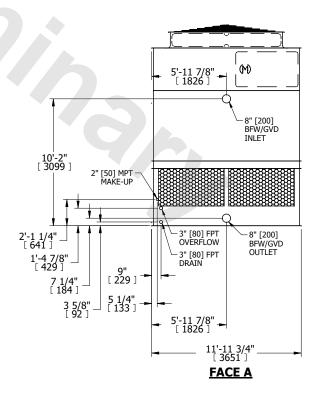
SHIPPING WEIGHT 8360 lbs+ [3795] kg+ OPERATING WEIGHT 14570 lbs+ [6610] kg+ HEAVIEST SECTION WEIGHT 5960 lbs+ [2705] kg+ NO. OF SHIPPING SECTIONS 2 DRAWN BY: KDS
