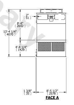
SHIPPING WEIGHT 8200 lbs+ [3720] kg+ OPERATING WEIGHT 13040 lbs+ [5915] kg+ HEAVIEST SECTION WEIGHT 2760 lbs+ [1255] kg+ NO. OF SHIPPING SECTIONS 4 DRAWN BY: JLG
