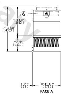
SHIPPING WEIGHT 9660 lbs+ [4385] kg+ OPERATING WEIGHT 15340 lbs+ [6960] kg+ HEAVIEST SECTION WEIGHT 3290 lbs+ [1495] kg+
