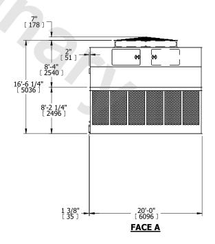
SHIPPING WEIGHT 23760 lbs+ [10780] kg+ OPERATING WEIGHT 44560 lbs+ [20215] kg+ HEAVIEST SECTION WEIGHT 7260 lbs+ [3295] kg+ NO. OF SHIPPING SECTIONS 4 DRAWN BY: BLL
