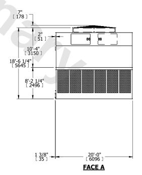
SHIPPING WEIGHT 27020 lbs+ [12260] kg+ OPERATING WEIGHT 47820 lbs+ [21695] kg+ HEAVIEST SECTION WEIGHT 8890 lbs+ [4035] kg+ NO. OF SHIPPING SECTIONS 4 DRAWN BY: KDS
