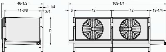
\*Capacity is based on a dry coil rating with R-717 at 1.2 : 1.0 recirculation rate with 35°F entering air temperature and 25°F saturated suction temperature.
