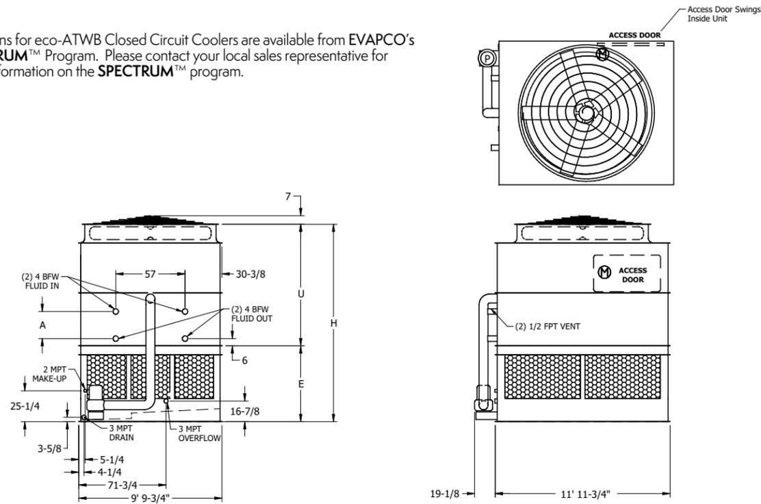
Note: The number of coil connections doubles when the flow rate exceeds 900 GPM on eco-ATW 10x12 models. This required option is referred to as the High Flow coil configuration.
