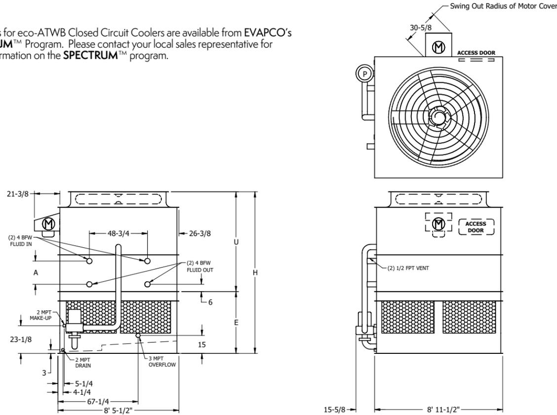
**Note:** The number of coil connections doubles when the flow rate exceeds 900 GPM on eco-ATW 9x9 models. This required option is referred to as the High Flow coil configuration.
