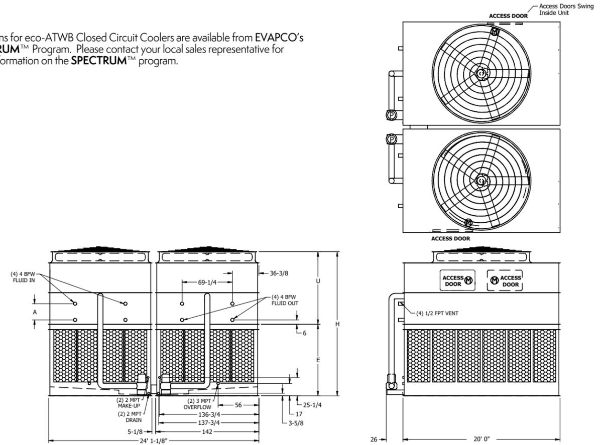
Note: The number of coil connections doubles when the flow rate exceeds 1,800 GPM on eco-ATW 24x20 models. This required option is referred to as the High Flow coil configuration.
