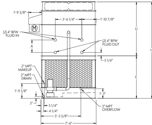
**Note:** The number of coil connections doubles when the flow rate exceeds 900 GPM on eco-ATWB 7x14 models. This required option is referred to as the High Flow coil configuration.
