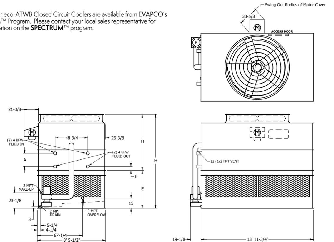
**Note:** The number of coil connections doubles when the flow rate exceeds 900 GPM on eco-ATW 9x14 models. This required option is referred to as the High Flow coil configuration.
