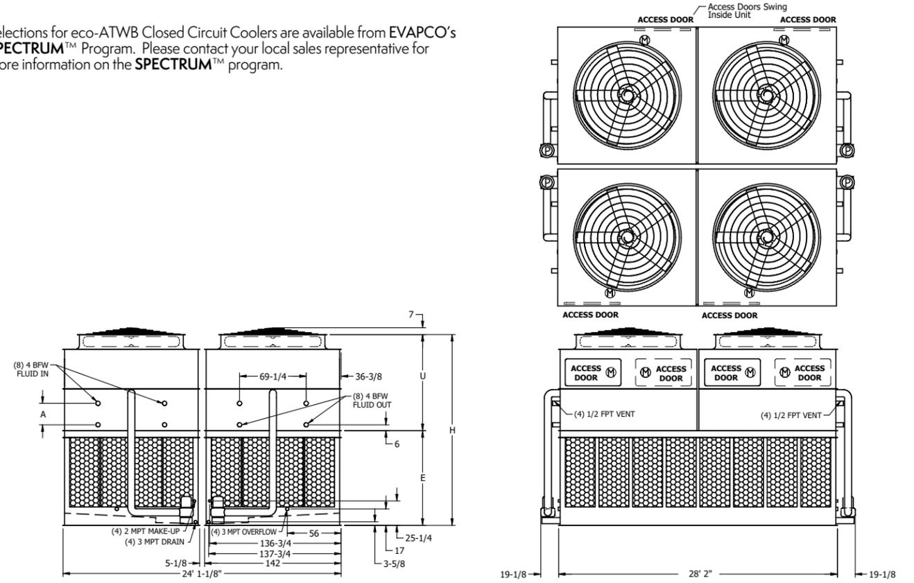
**Note:** The number of coil connections doubles when the flow rate exceeds 3,600 GPM on eco-ATW 24x28 models. This required option is referred to as the High Flow coil configuration.
