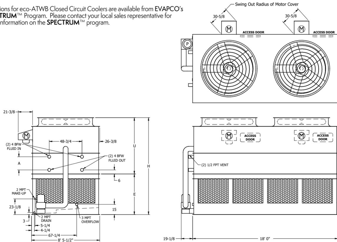
**Note:** The number of coil connections doubles when the flow rate exceeds 900 GPM on eco-ATW 9x18 models. This required option is referred to as the High Flow coil configuration.
