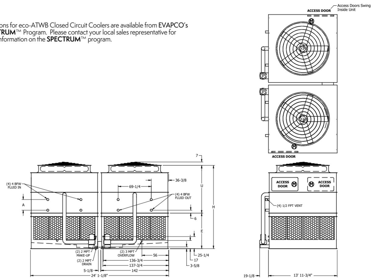
Note: The number of coil connections doubles when the flow rate exceeds 1,800 GPM on eco-ATW 24x14 models. This required option is referred to as the High Flow coil configuration.
