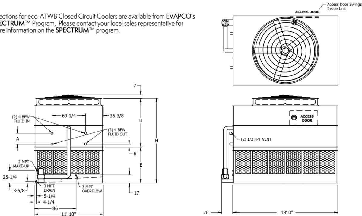
Note: The number of coil connections doubles when the flow rate exceeds 900 GPM on eco-ATW 12x18 models. This required option is referred to as the High Flow coil configuration.
