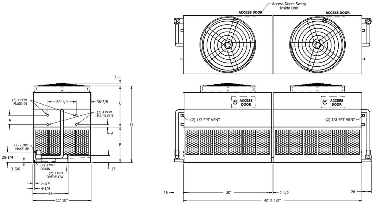
**Note:** The number of coil connections doubles when the flow rate exceeds 1,800 GPM on eco-ATW 12x40 models. This required option is referred to as the High Flow coil configuration.
