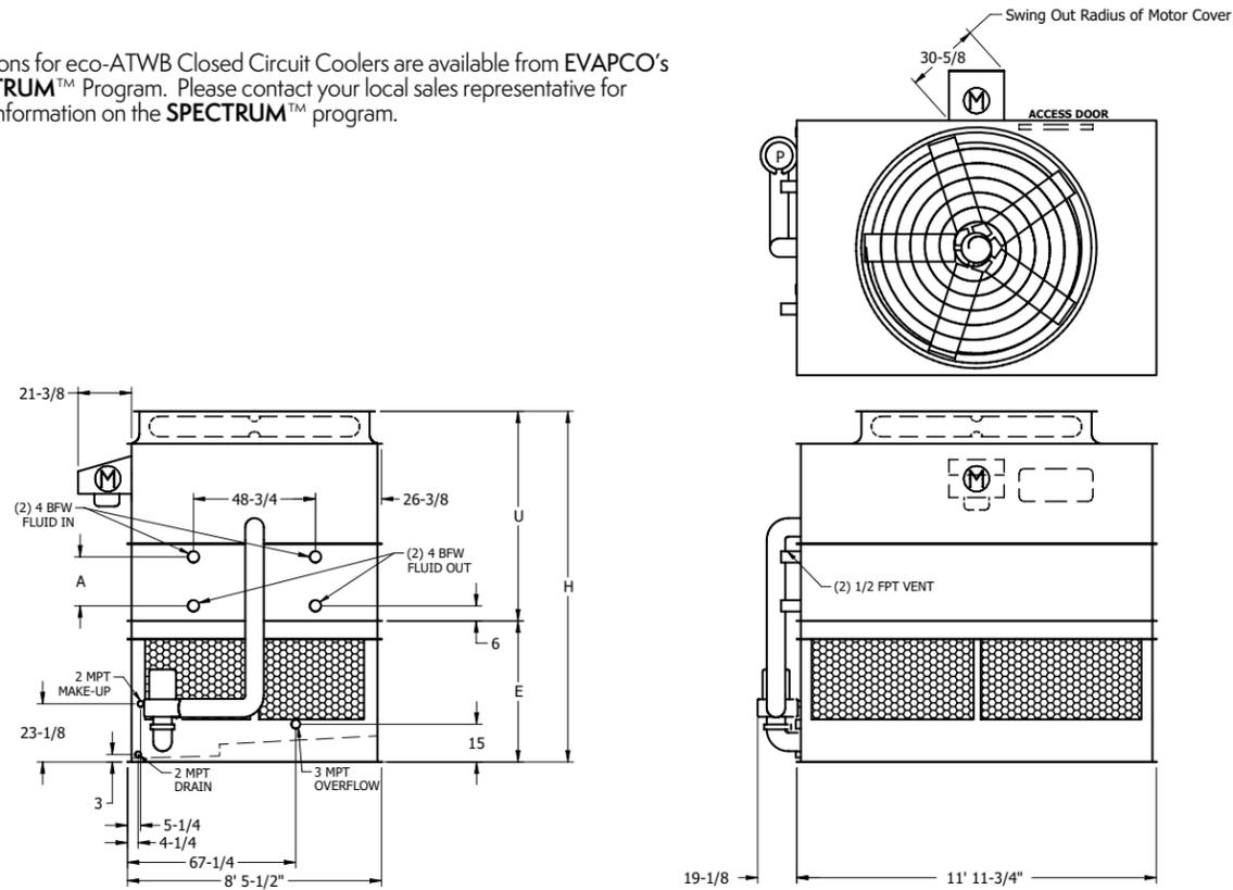
**Note:** The number of coil connections doubles when the flow rate exceeds 900 GPM on eco-ATW 9x12 models. This required option is referred to as the High Flow coil configuration.
