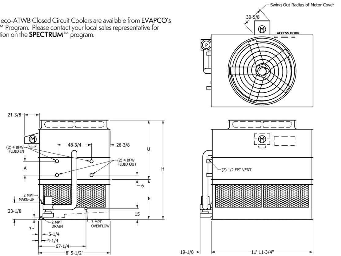
**Note:** The number of coil connections doubles when the flow rate exceeds 900 GPM on eco-ATW 9x11 models. This required option is referred to as the High Flow coil configuration.
