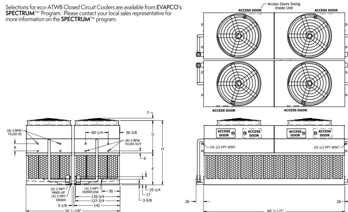
**Note:** The number of coil connections doubles when the flow rate exceeds 3,600 GPM on eco-ATC 24x40 models. This required option is referred to as the High Flow coil configuration.
