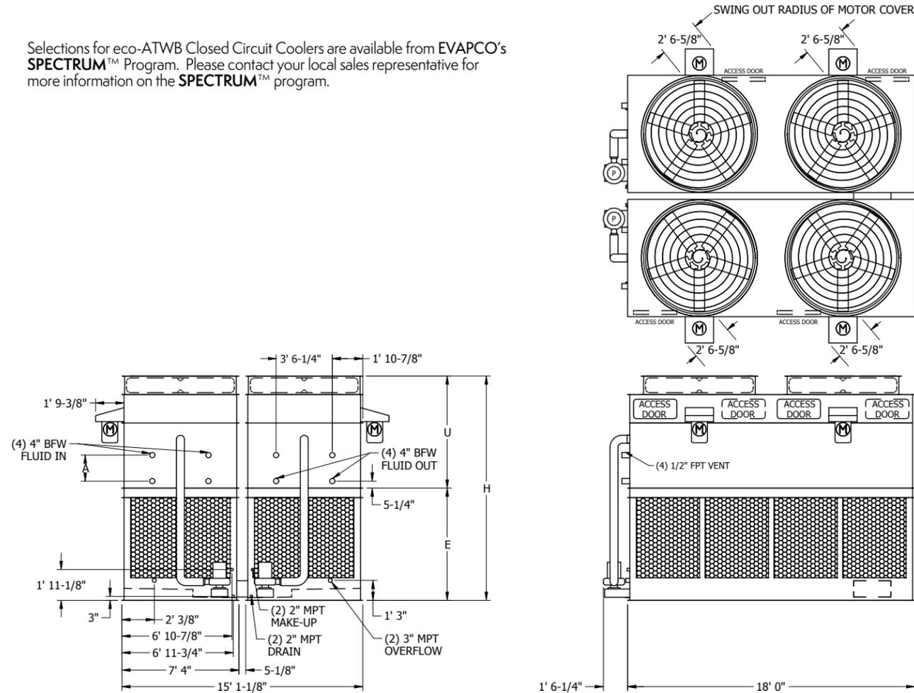
**Note:** The number of coil connections doubles when the flow rate exceeds 1,800 GPM on eco-ATWB 14x18 models. This required option is referred to as the High Flow coil configuration.
