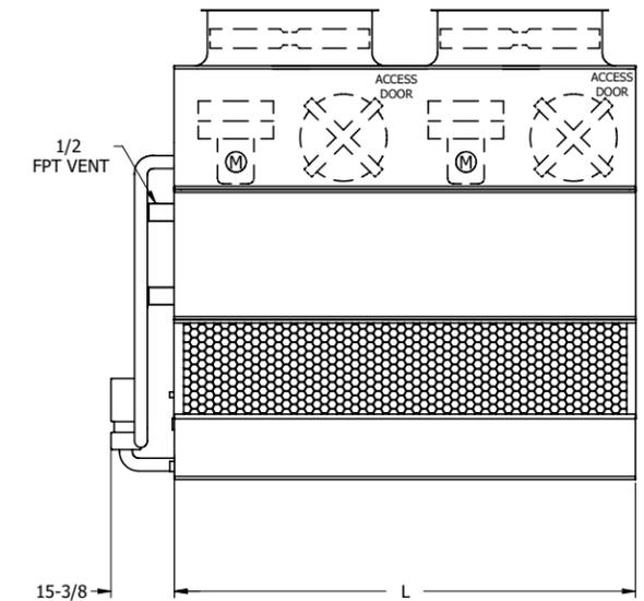
**Note:** The number of coil connections doubles when the flow rate exceeds 450 GPM on eco-ATW 4x9 and 4x12 models. This required option is referred to as the High Flow coil configuration.
