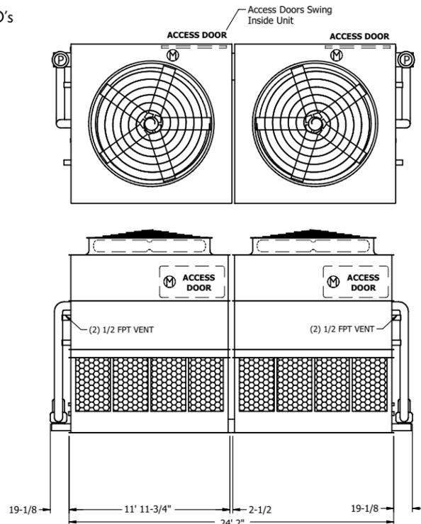
**Note:** The number of coil connections doubles when the flow rate exceeds 1,800 GPM on eco-ATW 12x24 models. This required option is referred to as the High Flow coil configuration.
