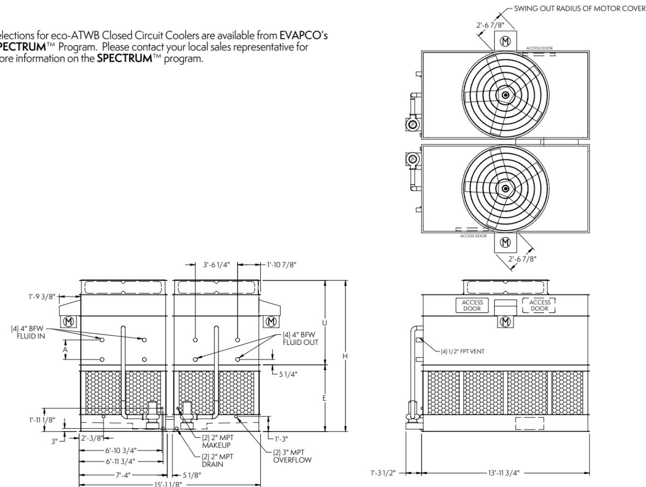
**Note:** The number of coil connections doubles when the flow rate exceeds 1,800 GPM on eco-ATWB 14x14 models. This required option is referred to as the High Flow coil configuration.
