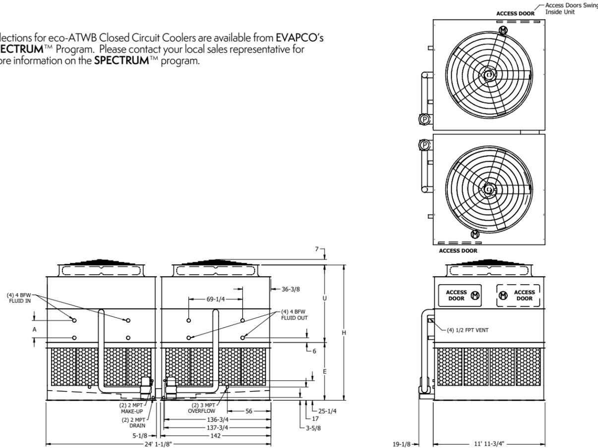
Note: The number of coil connections doubles when the flow rate exceeds 1,800 GPM on eco-ATW 24x12 models. This required option is referred to as the High Flow coil configuration.
