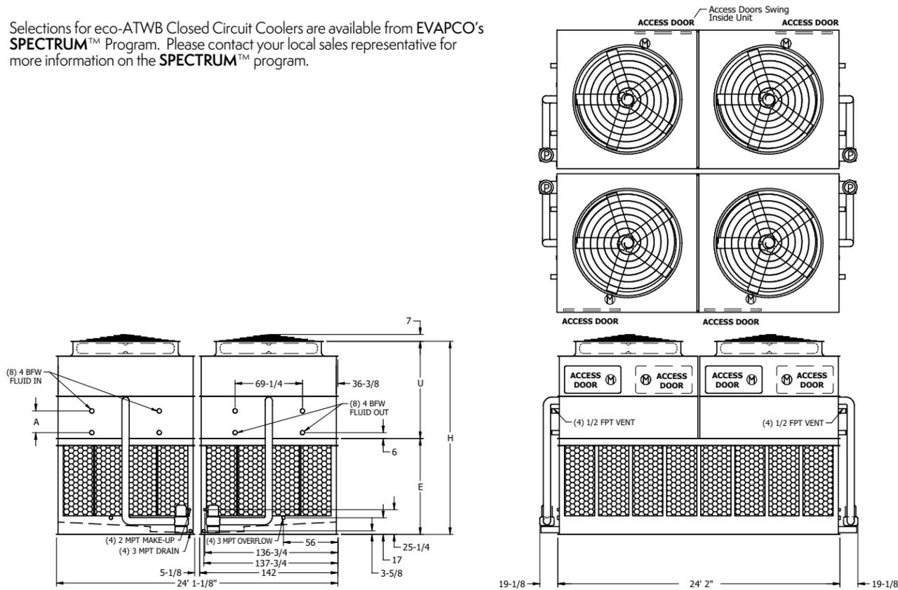
**Note:** The number of coil connections doubles when the flow rate exceeds 3,600 GPM on eco-ATW 24x24 models. This required option is referred to as the High Flow coil configuration.
