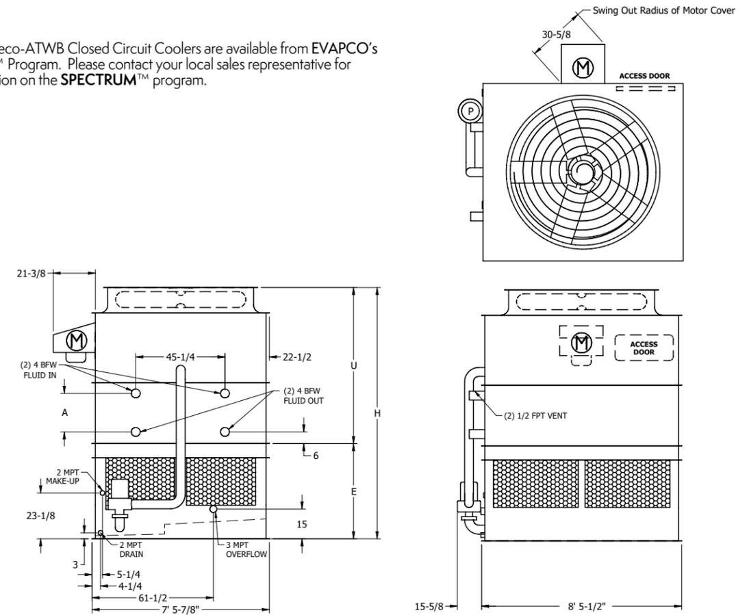
**Note:** The number of coil connections doubles when the flow rate exceeds 900 GPM on eco-ATW 9x8 models. This required option is referred to as the High Flow coil configuration.
