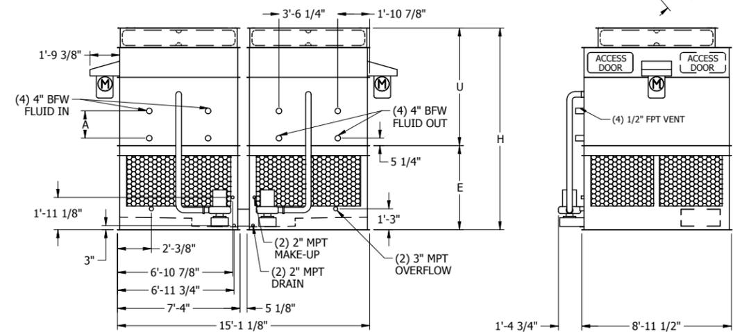
**Note:** The number of coil connections doubles when the flow rate exceeds 1,800 GPM on eco-ATWB 14x9 models. This required option is referred to as the High Flow coil configuration.
