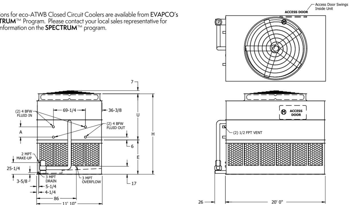
Note: The number of coil connections doubles when the flow rate exceeds 900 GPM on eco-ATW 12x20 models. This required option is referred to as the High Flow coil configuration.
