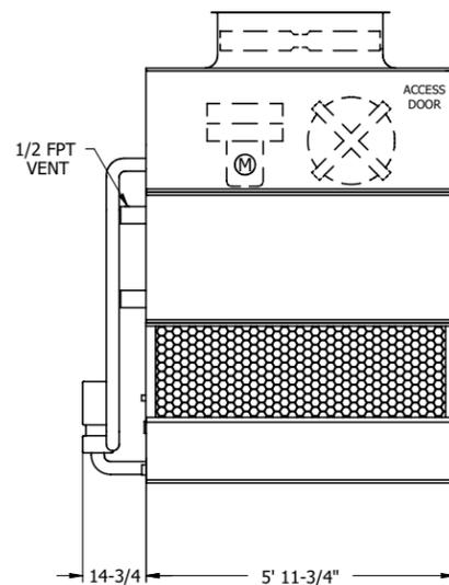
**Note:** The number of coil connections doubles when the flow rate exceeds 450 GPM on 4x6 models. This required option is referred to as the High Flow coil configuration.
