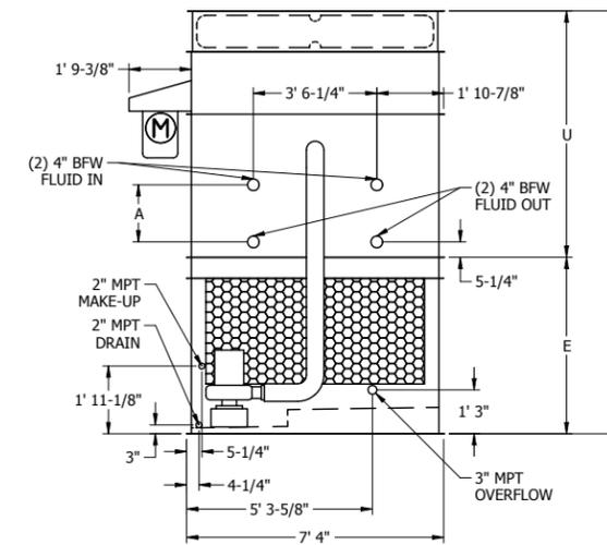
**Note:** The number of coil connections doubles when the flow rate exceeds 900 GPM on eco-ATWB 7x18 models. This required option is referred to as the High Flow coil configuration.
