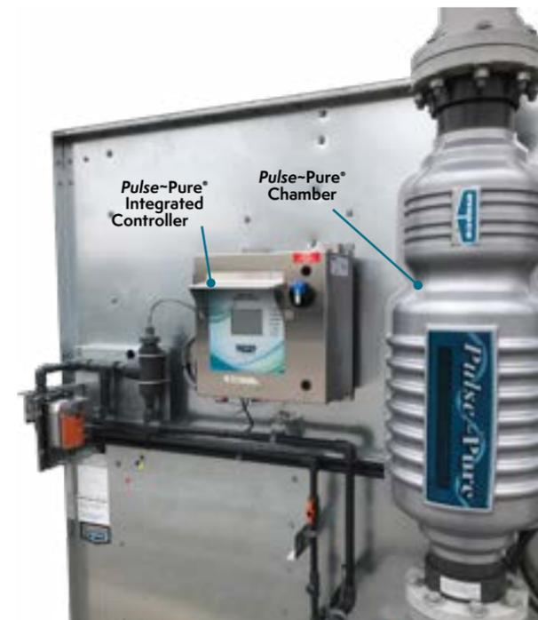
EVAPCO's Pulse~Pure® water treatment system utilizes pulsed electric field technology to provide an environmentally responsible alternative for the treatment of water in evaporative cooling equipment. The Pulse~Pure® system delivers short low- and high-frequency bursts of electromagnetic fields to the recirculating water in the fluid cooler.
