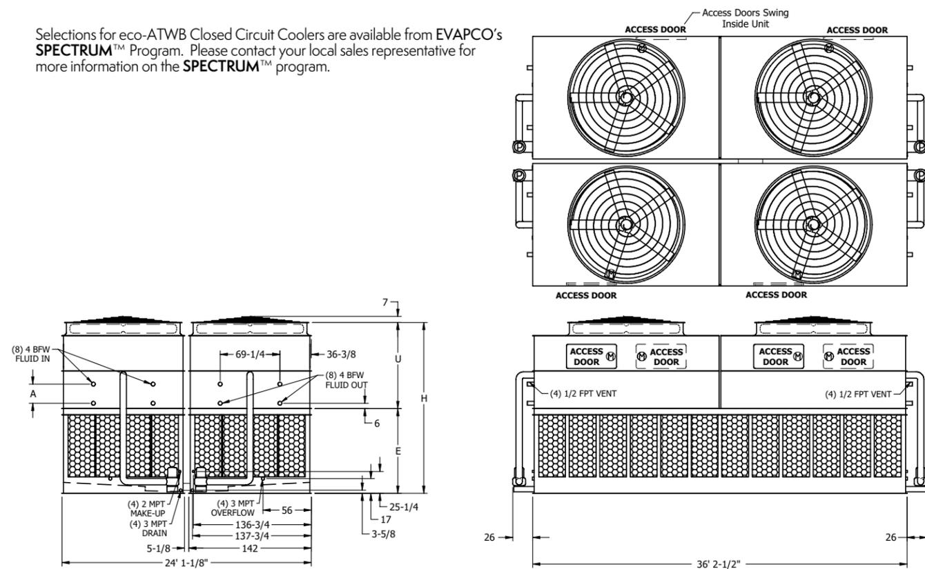
**Note:** The number of coil connections doubles when the flow rate exceeds 3,600 GPM on eco-ATW 24x36 models. This required option is referred to as the High Flow coil configuration.
