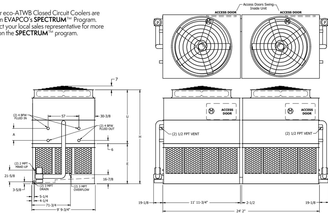
Note: The number of coil connections doubles when the flow rate exceeds 1,800 GPM on eco-ATW 10x24 models. This required option is referred to as the High Flow coil configuration.
