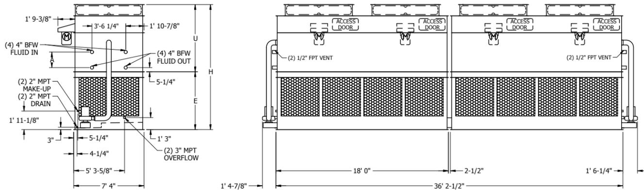
**Note:** The number of coil connections doubles when the flow rate exceeds 1,800 GPM on eco-ATWB 7x36 models. This required option is referred to as the High Flow coil configuration.
