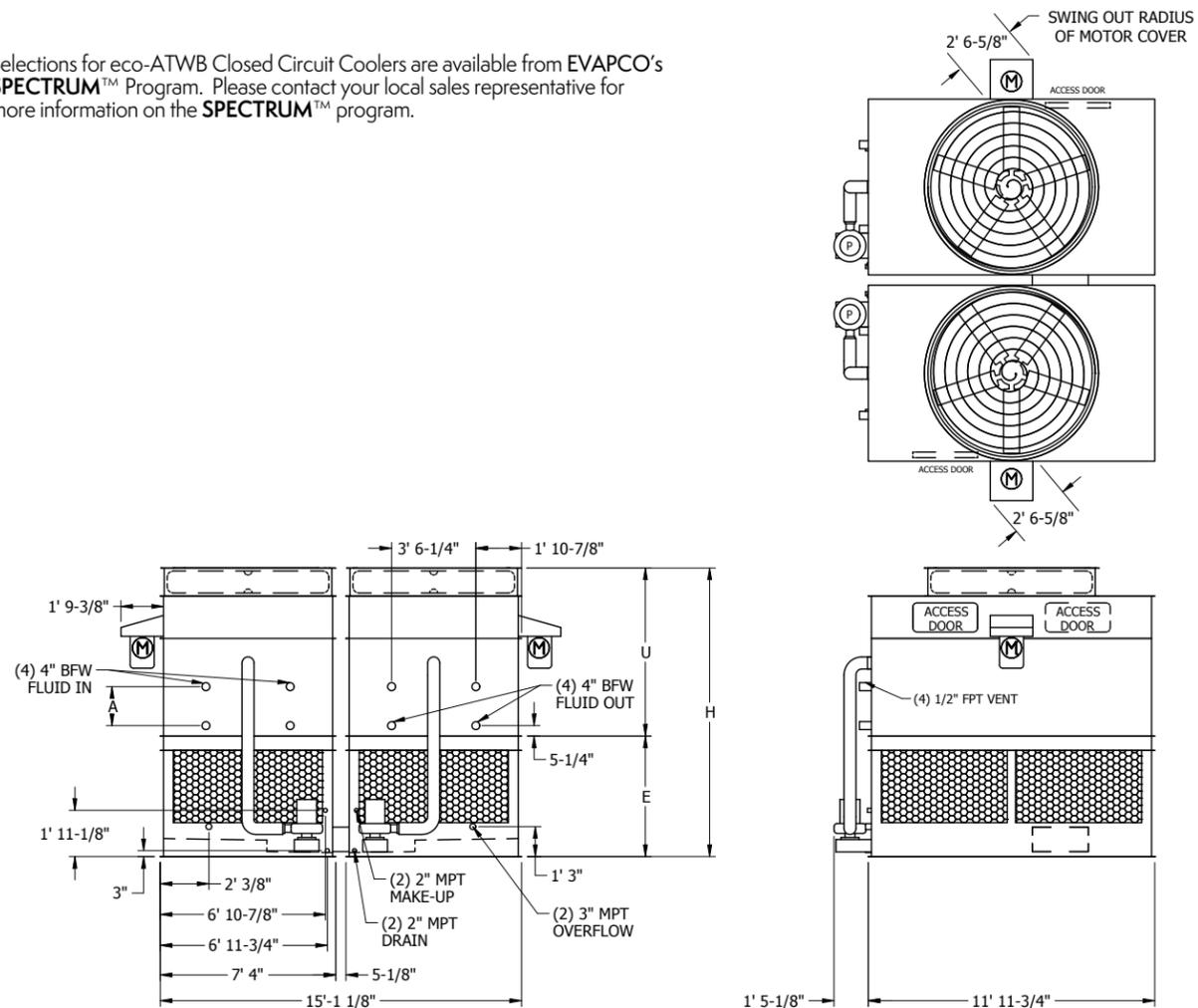
**Note:** The number of coil connections doubles when the flow rate exceeds 1,800 GPM on eco-ATWB 14x12 models. This required option is referred to as the High Flow coil configuration.
