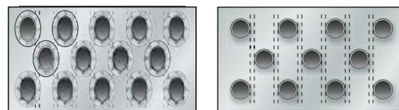
EVAPCO's Ellipti-fin® Finned Elliptical Tube
