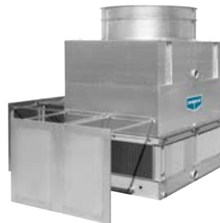
Electric immersion heaters can be added to the basin of your eco-ATWB closed circuit cooler. They are sized to maintain a +40° F (4.5° C) pan water temperature with the fans and system pumps off. A thermostat and low-water protection device cycle the heater on when required and prevent the heater elements from energizing unless they are completely submerged. All components are protected by rugged, weatherproof enclosures for outdoor use.
