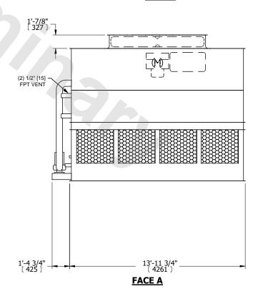
DRAWN BY: JLG NO. OF SHIPPING SECTIONS **SHIPPING** OPERATING HEAVIEST SECTION 13510 lbs+ [6130] kg+ 19810 lbs+ [8990] kg+ 11430 lbs+ [5185] kg+ WEIGHT WEIGHT WEIGHT
