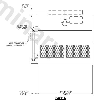
DRAWN BY: JLG NO. OF SHIPPING SECTIONS **SHIPPING** OPERATING HEAVIEST SECTION 10030 lbs+ [4550] kg+ 11900 lbs+ [5400] kg+ 17330 lbs+ [7865] kg+ WEIGHT WEIGHT WEIGHT
