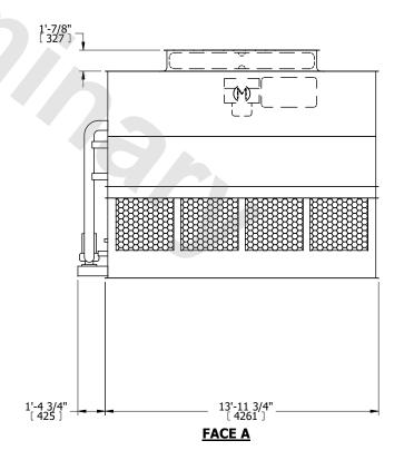
NO. OF SHIPPING SECTIONS **SHIPPING** OPERATING HEAVIEST SECTION 13500 lbs+ [6125] kg+ 18200 lbs+ [8260] kg+ 11420 lbs+ [5185] kg+ WEIGHT WEIGHT WEIGHT
