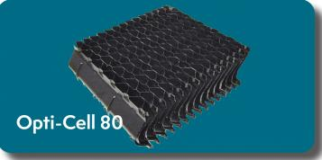
The OC-80 is a high-efficiency drift eliminator for counterflow cooling towers. Made from durable, corrugated PVC, it resists UV, rot, fungi, bacteria, solvents, acids, alkalis, and common cooling tower chemicals.
