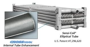
The coils are manufactured from high quality steel tubing following the most stringent quality control procedures. Each circuit is inspected to ensure the material quality and then tested before being assembled into a coil. Finally, the assembled coil is pneumatically tested at 390 psig under water to ensure it is leak free.
