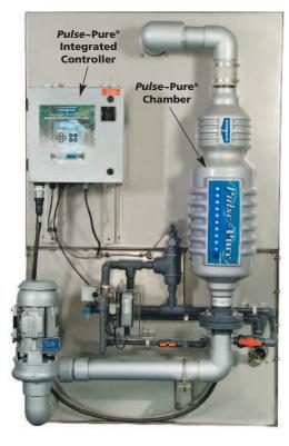
EVAPCO's *Pulse*~Pure\* water treatment system utilizes pulsed electric field technology to provide an environmentally responsible alternative for the treatment of water in evaporative cooled equipment. The *Pulse*~Pure\* system delivers short, high-frequency bursts of low energy electromagnetic fields to the recirculating water in the ESWB.
