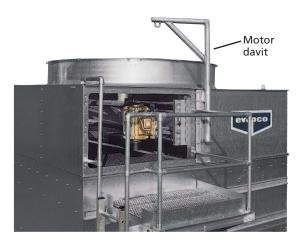
The economical motor davit option eliminates the need for a crane in the event that a fan or motor needs to be removed. The service mechanic only needs a chain-fall or come-along for easy removal of these items. The motor davit is constructed from heavy duty aluminum with easy mounting to the unit in the field.
