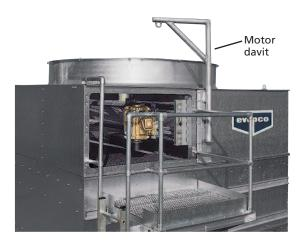
The motor davit option is an economical option which eliminates the need for a crane in the event that a fan motor has to be removed. The service mechanic only needs a chain-fall or come-along for easy removal of these heavy items. The motor davit is constructed from heavy duty aluminum with easy mounting to the unit in the field.
