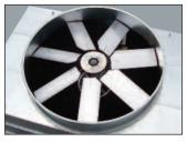
sound levels are desired. Low Sound Fan construction uses aluminum blades and a steel fan hub. The Low Sound Fan is capable of reducing the unit sound pressure levels by **4 dB(A) to 7dB(A)**, depending on specific unit selection and measurement location
