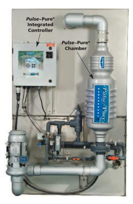
EVAPCO's *Pulse*~**Pure**<sup>®</sup> water treatment system utilizes pulsed electric field technology to provide an environmentally responsible alternative for the treatment of water in evaporative cooled equipment. The *Pulse*~**Pure**<sup>®</sup> system delivers short, high-frequency bursts of low energy electromagnetic fields to the recirculating water in the ESWA.
