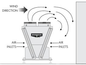
**Figure 1-** Effect of Wind Directed Toward Surrounding Structure when Top of Unit is Lower Than Adjacent Structure
