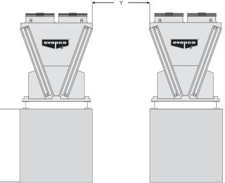
Figure 9 – V-Coil & Double Stack Model Elevation and Spacing Positions
