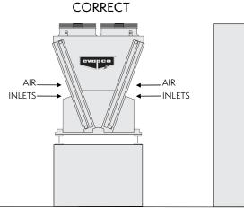
Figure 3- Elevated Installation so Top of Unit is Level with or Higher than Adjacent Structure
