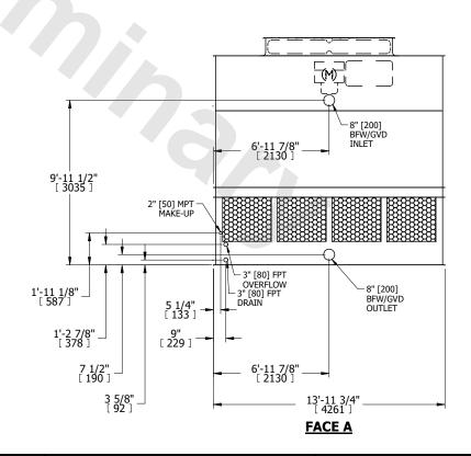
SHIPPING WEIGHT 6700 lbs+ [3040] kg+ OPERATING WEIGHT 11210 lbs+ [5085] kg+ HEAVIEST SECTION 4650 lbs+ [2110] kg+
