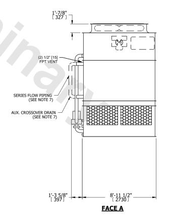
DRAWN BY: JLG NO. OF SHIPPING SECTIONS **SHIPPING** OPERATING HEAVIEST SECTION 11760 lbs+ [5335] kg+ 13200 lbs+ [5990] kg+ 18860 lbs+ [8555] kg+ WEIGHT WEIGHT WEIGHT
