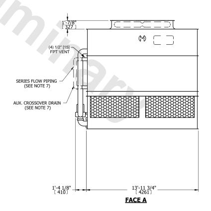
DRAWN BY: JLG NO. OF SHIPPING SECTIONS **SHIPPING** OPERATING HEAVIEST SECTION 19280 lbs+ [8750] kg+ 21360 lbs+ [9690] kg+ 29640 lbs+ [13445] kg+ WEIGHT WEIGHT WEIGHT
