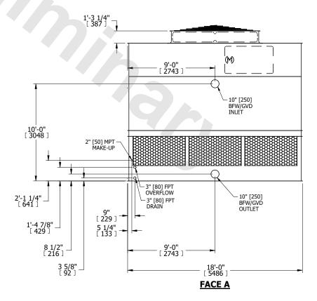
SHIPPING WEIGHT 10680 lbs+ [4845] kg+ OPERATING WEIGHT 18280 lbs+ [8295] kg+ HEAVIEST SECTION WEIGHT 7130 lbs+ [3235] kg+ NO. OF SHIPPING SECTIONS 2 DRAWN BY: KDS
