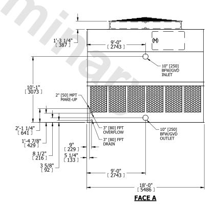
DRAWN BY: KDS NO. OF SHIPPING SECTIONS **SHIPPING** OPERATING HEAVIEST SECTION 11860 lbs+ [5380] kg+ 21130 lbs+ [9585] kg+ 7960 lbs+ [3615] kg+ WEIGHT WEIGHT WEIGHT
