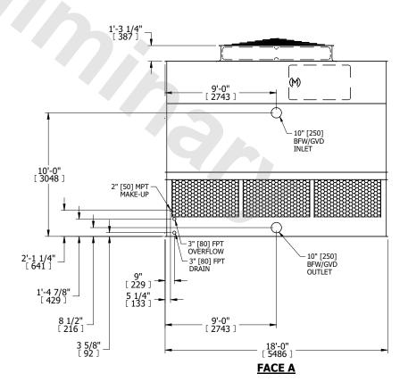
**SHIPPING** OPERATING HEAVIEST SECTION 10780 lbs+ [4890] kg+ 18380 lbs+ [8340] kg+ 7230 lbs+ [3280] kg+ WEIGHT WEIGHT WEIGHT
