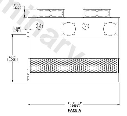
SHIPPING WEIGHT 2570 lbs+ [1170] kg+ OPERATING WEIGHT 4690 lbs+ [2130] kg+ HEAVIEST SECTION WEIGHT 1810 lbs+ [825] kg+ NO. OF SHIPPING SECTIONS 2 DRAWN BY: KWC
