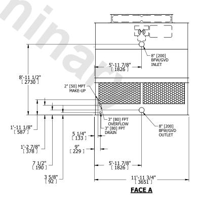
SHIPPING WEIGHT 5580 lbs+ [2535] kg+ OPERATING WEIGHT 9440 lbs+ [4285] kg+ HEAVIEST SECTION WEIGHT 3820 lbs+ [1735] kg+ NO. OF SHIPPING SECTIONS 2 DRAWN BY: JLG
